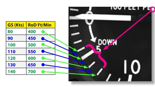
NOTE The range of 3° RoD's for the speeds from 80-140Kts is represented by a very tight range on the VSI display of just 300'/min.
