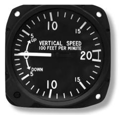
In reality the most accurate RoD you can probably fly to is +/- 50'/min, so keep the flying and the maths simple as well.
